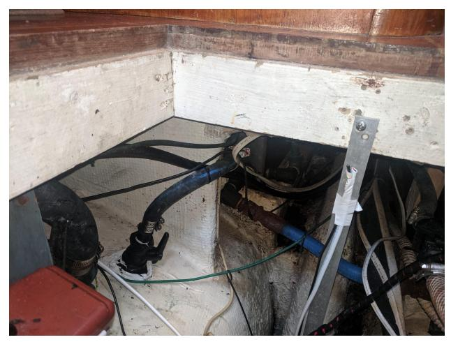
The structural grid is glassed to the hull. In some places the grid reinforced by bulkheads that extend down to the hull (one of which is pictured).
