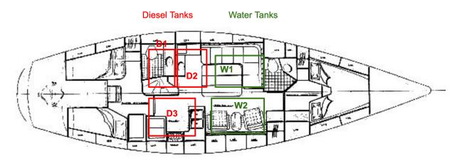
D1 and D2 - D1 starts under head and D2 ends at port setee start - wouldn't know they're separate except the separate fills & valved hose joining them
